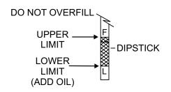
Figure 21. Engine Oil Check
